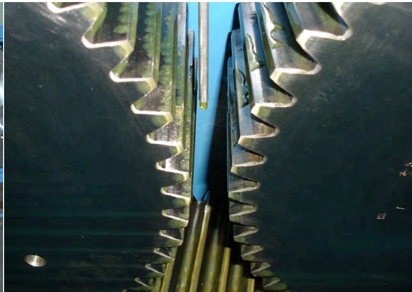
Hardened and ground helical gears
