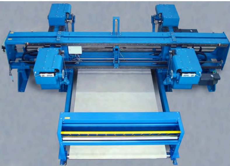
Dual centre driven Let-Off station with automatic fabric centring
