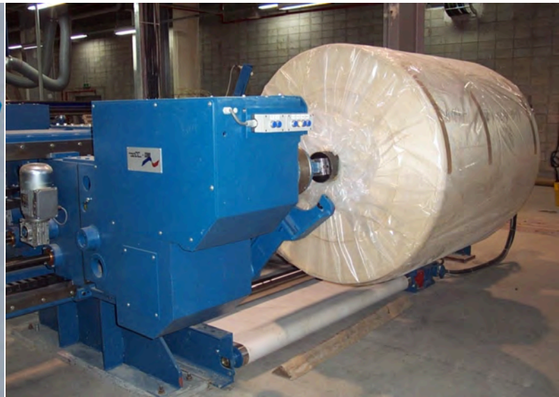
Dual centre driven Let-Off station with generating motor brake
